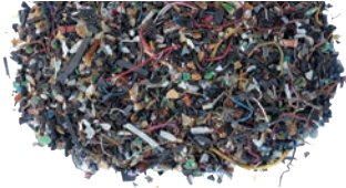
Gold, silver, and copper sediment sludge (mixed metal)
