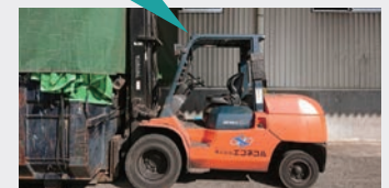
Forklift with drive recorder
