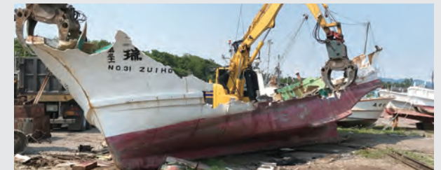
Dismantling of vessels
